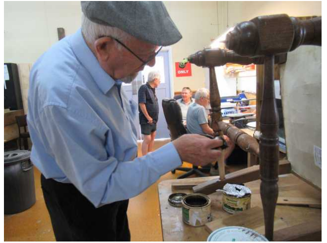
David McKenzie turned and fitted two chair stretchers. Picture two shows him staining the new parts to match the original.
